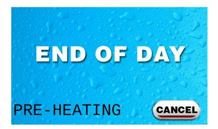
After reaching 350 degrees it will run for 25 minutes removing any residual moisture from the unit. You can cancel at any time to return to the main menu screen.
